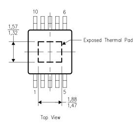
NOTE: All linear dimensions are in millimeters
